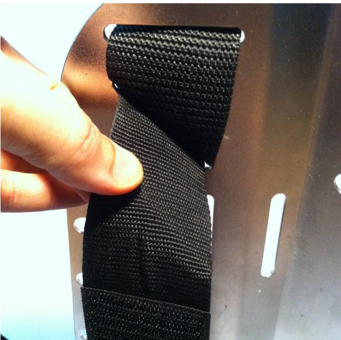
3 - Run the top of the mounting strap through the lower angled slot of your back plate. The exact position of these slots will affect how far from your body center line the counter lungs will be.
