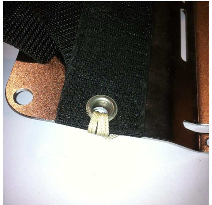
2 - Secure the included mounting strap, Velcro facing outwards, to the hole close to the harness slots of your back plate with nylon line. 5-6 wraps will ensure the strap does not move sideways. Tie a square knot on the back side and melt the ends together. The exact position of the hole will affect the available volume of the counter lung. Some back plates do not have a hole at a suitable position. If you need to drill a hole, make sure to deburr it.
