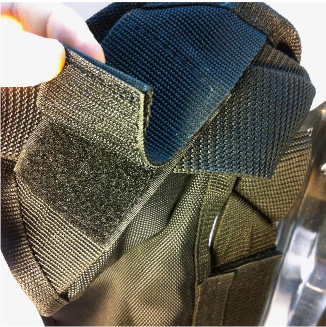
8 – Attach the counter lungs so that the bottom of each lung is aligned with the bottom edge of the back plate as a starting point. Close the top Velcro straps so that the mating Velcro patches are perfectly aligned. If not aligned it will either restrict the volume or make the lung float above your shoulder.
