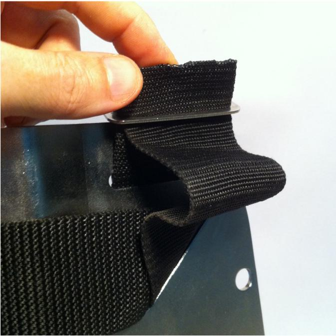
4 – Feed the mounting strap through the 3-bar slide and pull it tight.
