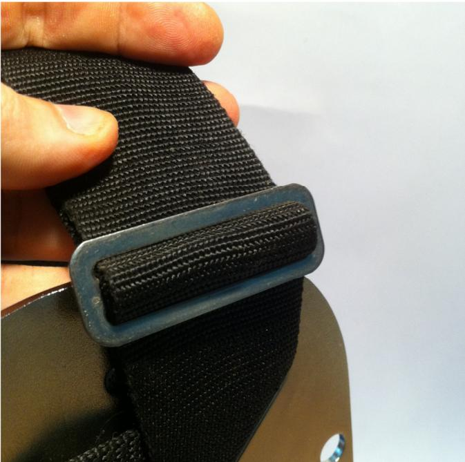
6 – The slide should sit close to the top edge of your back plate. Check that the mounting strap is tight when you pull the harness upwards like when wearing the back plate. The strap needs to be tight to prevent side to side movement of the counter lung.
