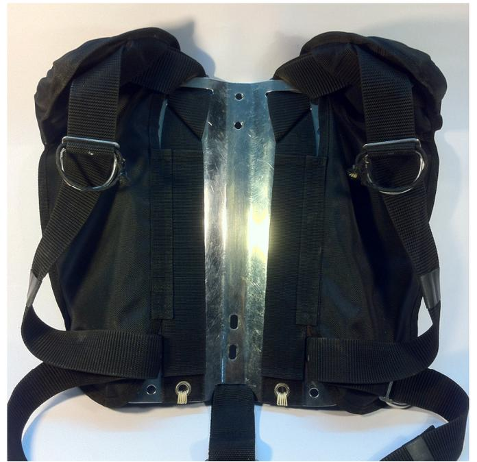
9 – Final adjustments of side to side position and height will have to be determined during actual dives. The picture shows a good starting point. If the back plate is worn low on your back you may have to move the counter lungs higher on the back plate. When the harness and counter lung height is properly adjusted the T-piece port will sit slightly behind the top of your shoulder.
